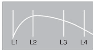
Fig.2 More crowning at the ends and tapering correction.
