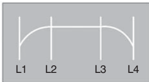
Fig.1 Crowning more stressed at the ends.
