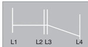
Fig.4 Double tapering or parallel plus conical.
